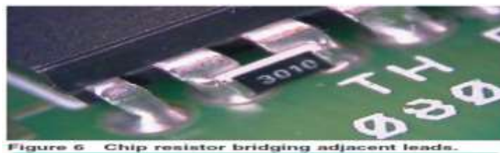
Figure 6 Chip resistor bridging adjacent leads.
